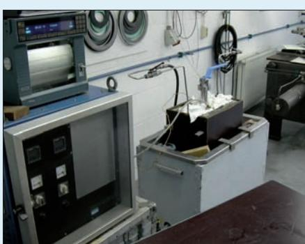
Typical set-up for testing a small valve.
