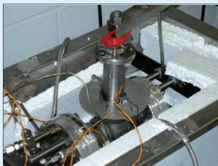
Valve being prepared for testing at DCI. Note the multiple thermocouples, used to obtain accurate temperature measurements at various parts of the valve.
