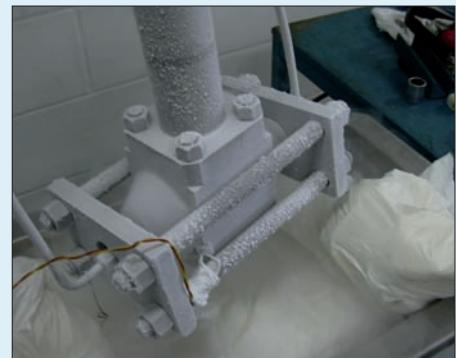
The rate at which a valve is cooled can be varied according to the needs of the client.
